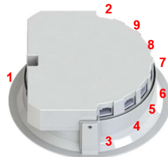
Figure 3 LiFiMAX AP with its recessed mounting accessory
